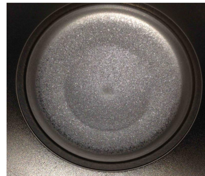
CoFeB sputtering target (Ø100mm)
