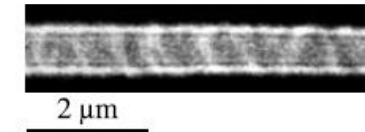
Fig. 2.26. Lorentz picture of a polycrystalline Permalloy film showing the streaky ripple texture perpendicular to the mean magnetization in the domains and cross-tie walls. The convergent wall displays diffraction fringes as shown in the enlargement. (Courtesy S. Tsukahara [261])
