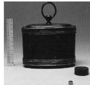
An early eighteenth century lodestone, a ferrite magnet (right) and a Nd-Fe-B magnet (front), which all store about a joule of energy.
