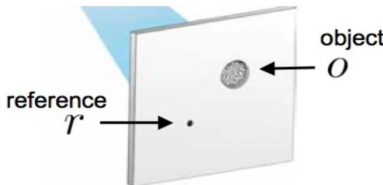
$$\begin{aligned} &= |\mathcal{F}\{r + o\}|^2 \\ &= |R + O|^2 \\ &= |R|^2 + |O|^2 + OR^* + RO^* \\ &\quad \mathcal{F}\{\text{Hologram Intensity}\} \\ &r * r + o * o + o * r + r * o \end{aligned}$$
