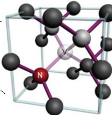
Single NV defect in diamond tip: magnetic sensor with an atomic size
