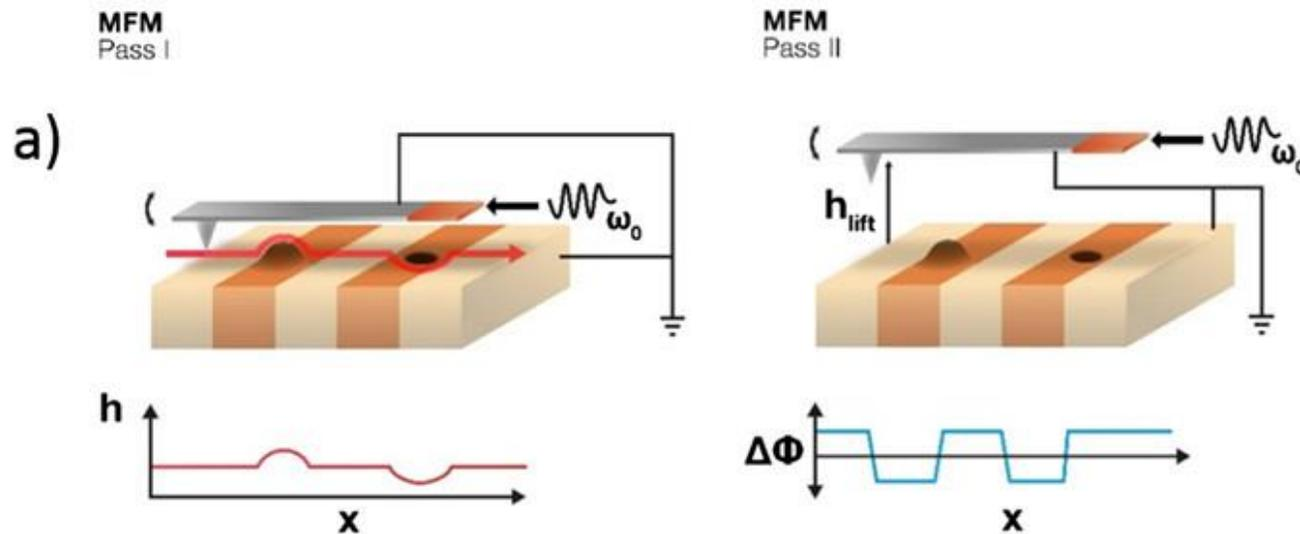
Tip: **dipole moving in a gradient of magnetic field**
