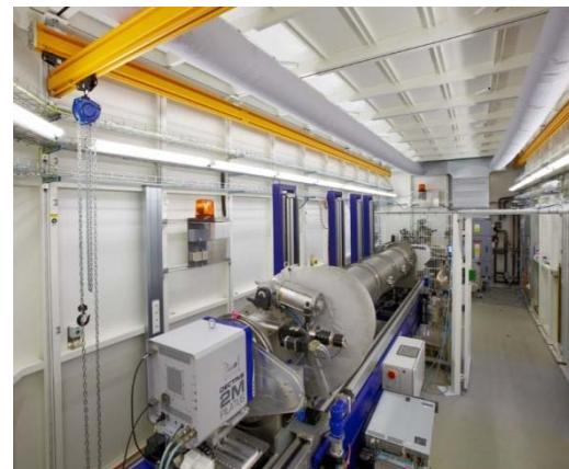
Variable sample to detector distance from 1.5 m to 6 m
