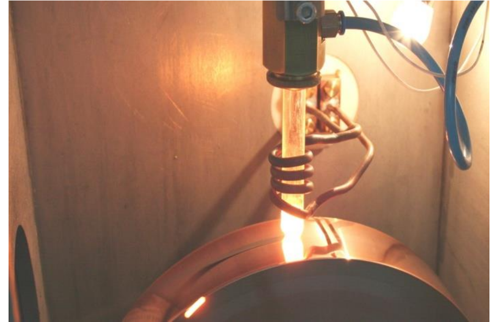
Rapidly quenching equipment for amorphous and nanocrystalline ribbons preparation.
