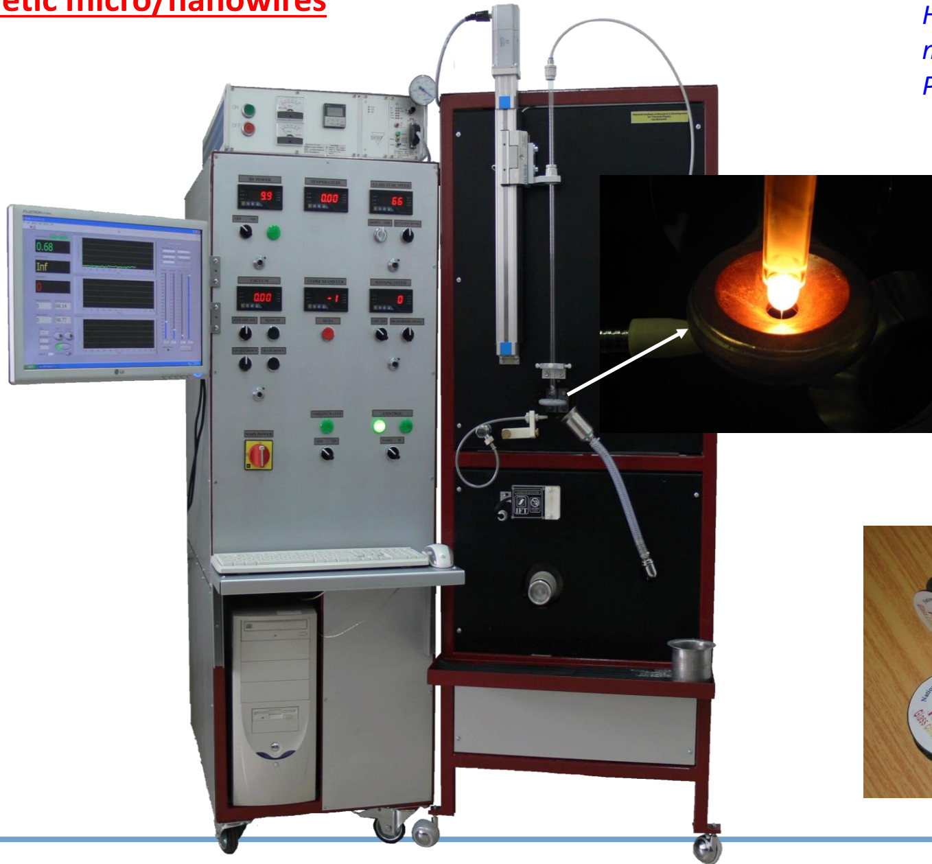
Glass-covered micro/nanowires preparation equipment.
