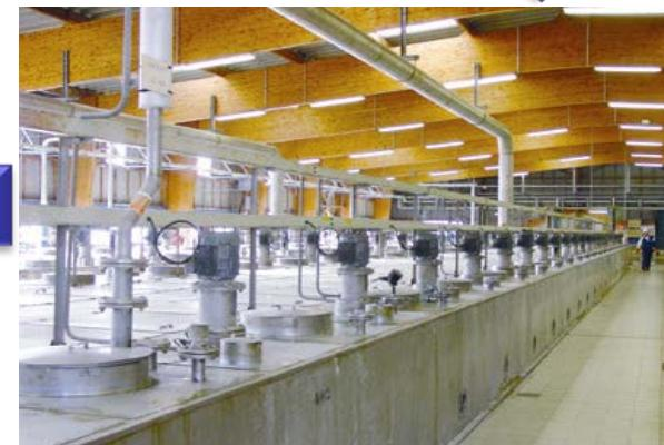
Solvent extraction is the only industrial process used commercially for REE separation
