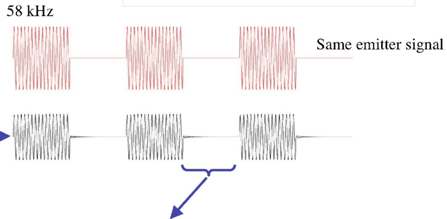
The receiver do not detect oscillations between pulses
