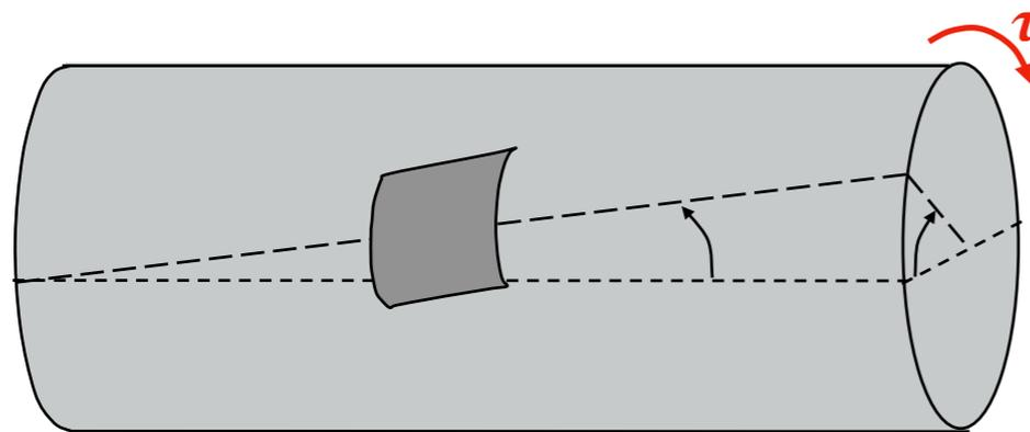
The torsion deforms the surface
