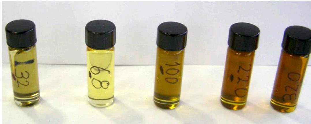
lubricant oils with different viscosities
