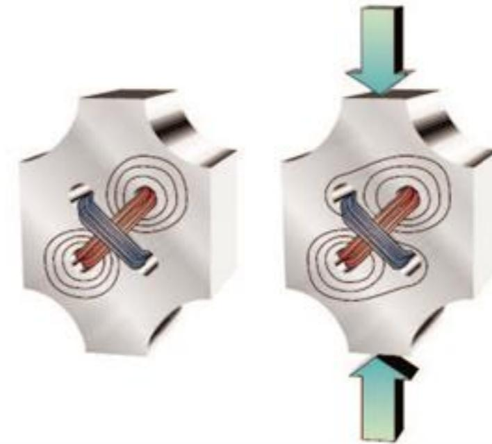
Pressductor force sensor (ABB)
