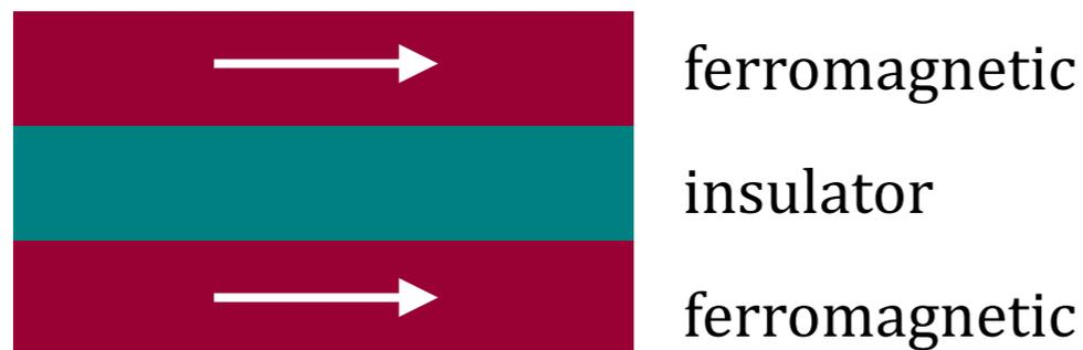
Magnetic Tunnel Junctions (MTJ) are composed of multiple layers
