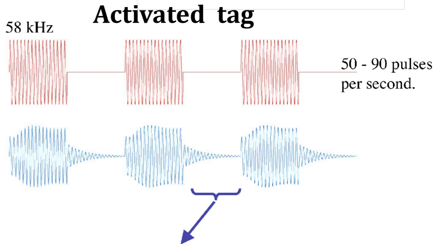
The emitter pulses **excite oscillations** that remain after the pulses end if the element is tuned to the pulses frequency
