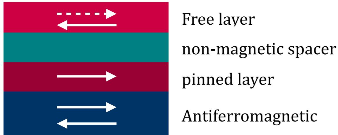
The free layer magnetization rotates in small field
