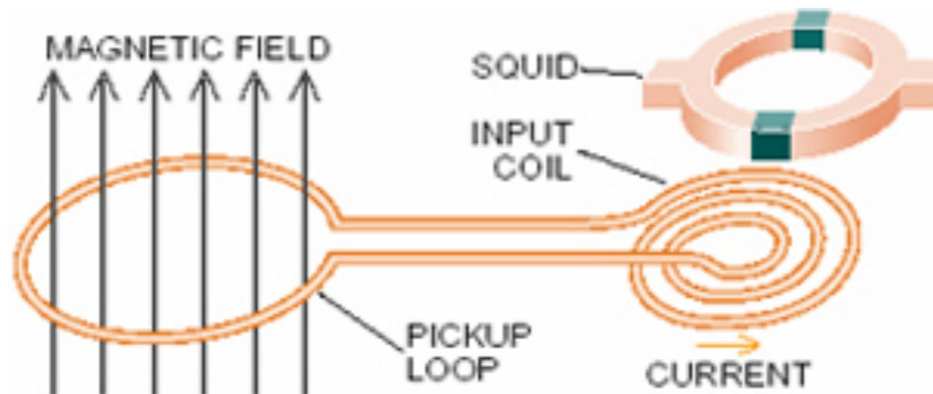
There are both ac and dc SQUIDS. Today they can also be made with high temperature superconductors.
