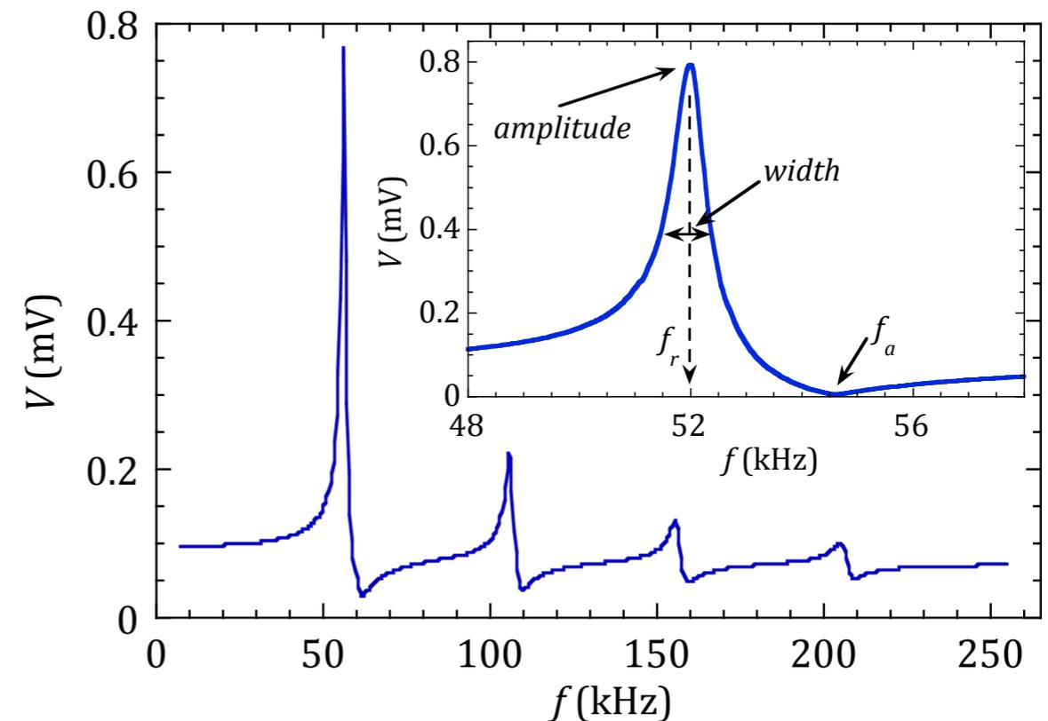
When the wavelength matches the length of the sample, standing waves build up, and resonance takes place.
