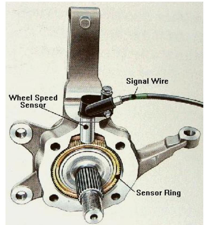
*Anti-lock Braking System (ABS)*
