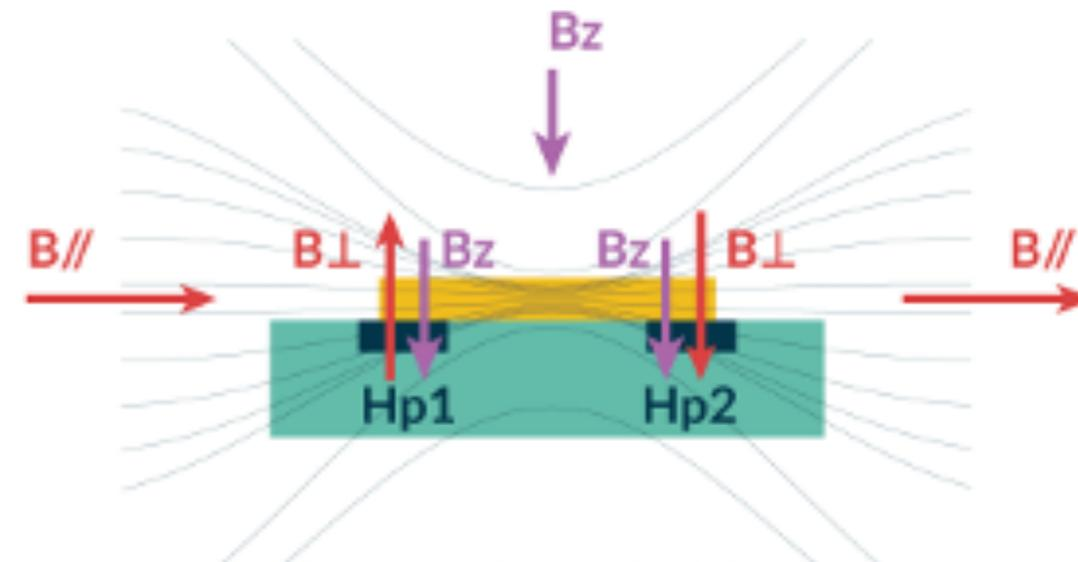
The in-plane fields develop perpendicular components
