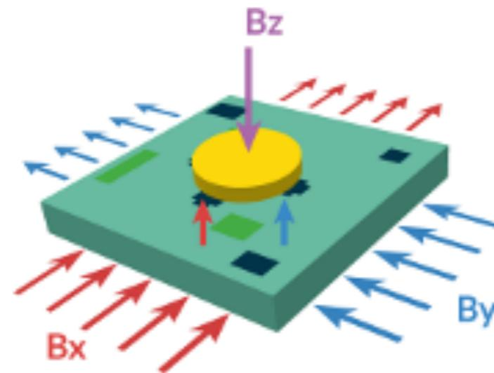
A magnetic concentrator (permalloy film) is deposited on top
