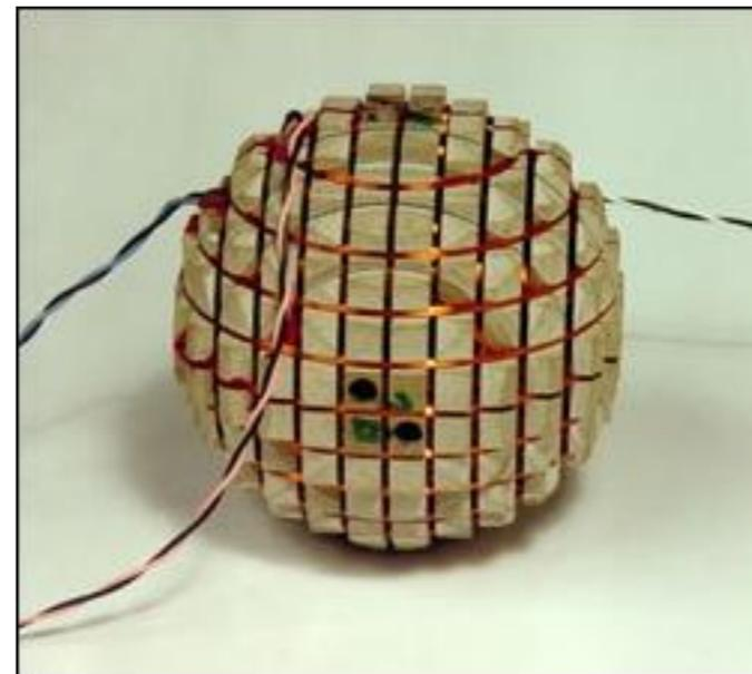
*fluxgate space magnetometer*
