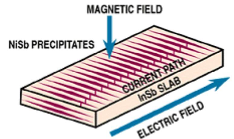
*Feldplatte* sensors, with traversal NiSb needles. Developed by Weiss (1966), commercialized by Siemens.
