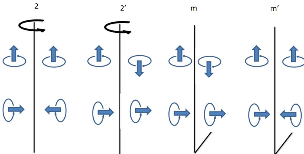
B. Magnetic moments on special Wyckoff positions have less degree of freedom. Examine the possible orientation of the moment of an atom on a 2 and  $2'$  fold-axis.
