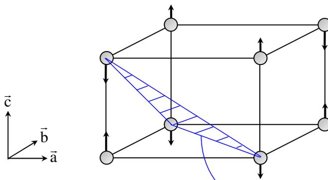
Doubling of the unit cell along a, b, and c, ferromagnetic planes perpendicular to  $\vec{a} + \vec{b} + \vec{c}$ ,  $\mathbf{k}=(1/2, 1/2, 1/2)$
