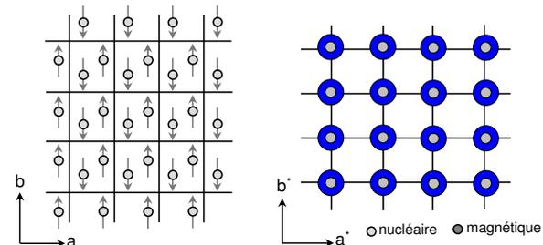
Antiferromagnetic  $k=(0, 0, 0)$ , 2 atoms per unit cell: no doubling of the unit cell but antiferromagnetic arrangement within the unit cell.
