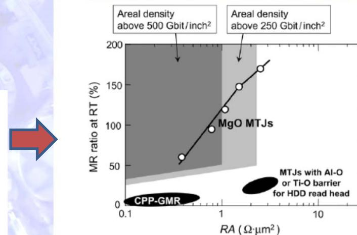
Figure 29. MR ratio at RT versus resistance-area (RA) product. Open circles are values for CoFeB/MgO/CoFeB MTJs. (Adapted from [46].) Light grey and dark grey areas are the zones required for HDDs with recording densities above 250 and 500 Gbit/inch<sup>2</sup>.
