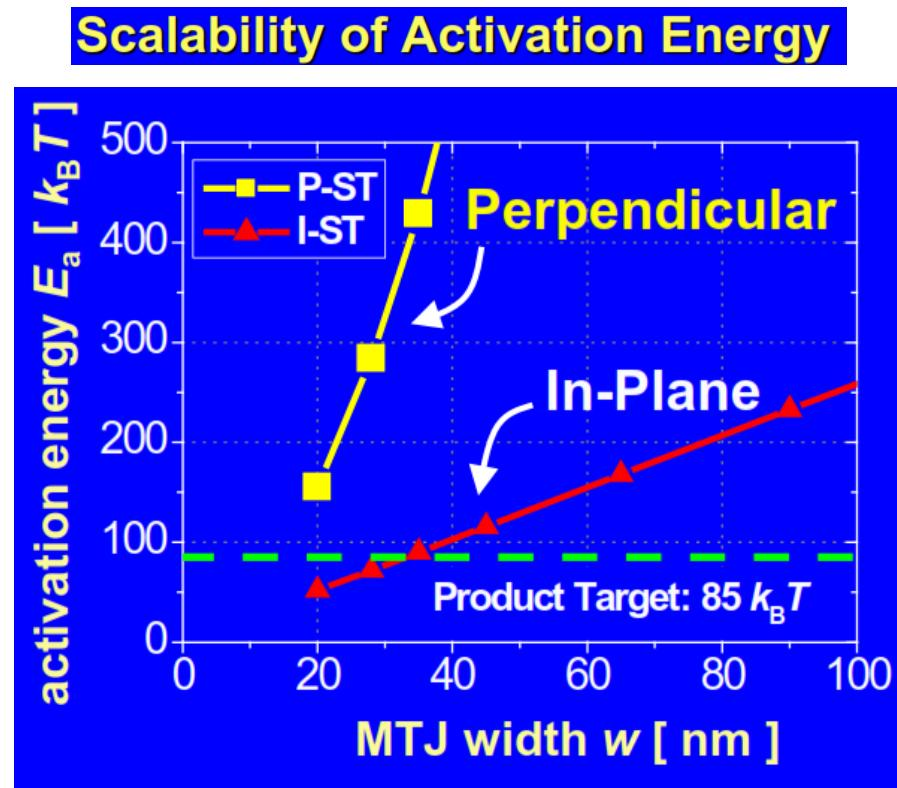
$$I_{C0} = \alpha \frac{\gamma e}{\mu_B g} M_s H_K V = 2\alpha \frac{\gamma e}{\mu_B g} E$$
