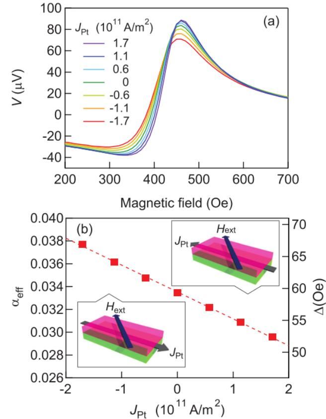
FIG. 2. (a) ST-FMR spectra for various dc's applied to Py (1.9 nm)/Pt (3.5 nm) sample with  $\theta = 45^\circ$ . (b)  $J_{\text{Pt}}$  dependence of  $\alpha_{\text{eff}}$  and  $\Delta$ .
