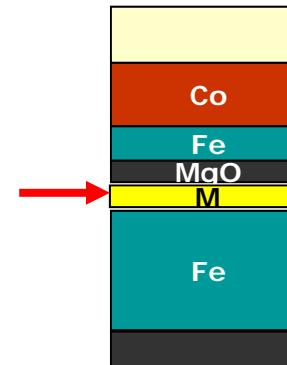
Giant tunneling magnetoresistance up to 410% at room temperature
