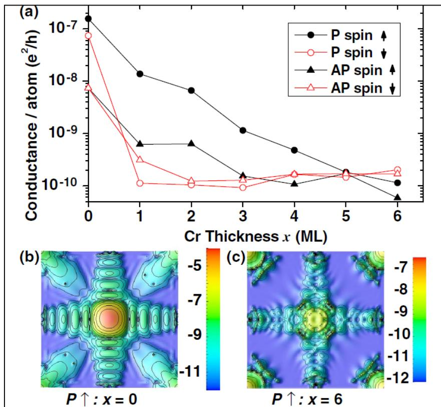
FIG. 3 (color online). Fe/Cr( $x$  ML)/MgO(10 ML)/Fe: (a) evolution of the P $\uparrow$ , P $\downarrow$ , AP $\uparrow$ , and AP $\downarrow$  conductance channels with increasing Cr thickness  $x$ . Transmission probability of the dominant P $\uparrow$  conductance channel as a function of  $k_{\parallel}$  for (b)  $x = 0$  and (c)  $x = 6$ .
