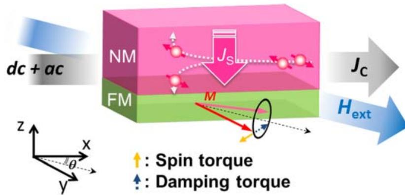
FIG. 1. Schematic illustration of SHE-induced EDM.  $J_s$  denotes spin current (density) due to dc inside Pt layer through SHE, which exerts spin transfer torque on magnetization inside FM layer and effectively reduces damping torque. The FMR spectrum can be detected as a dc voltage spectrum with applying an ac through the mixing of the ac and oscillatory change of anisotropic magnetoresistance.
