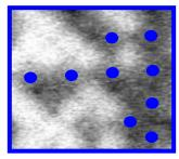
Mean switching field: 7200 Oe SFD ( $\sigma$ /mean) = 11.5 %
