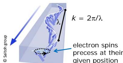
Solution of EoM for a thin film:
