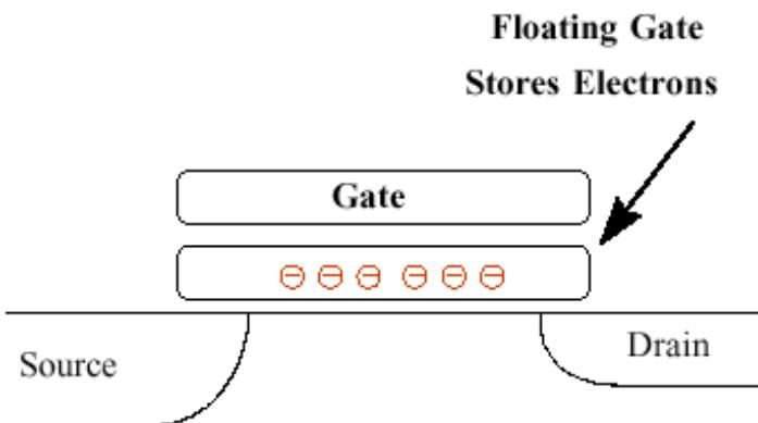
Figure 2: Single transistor flash memory cell
