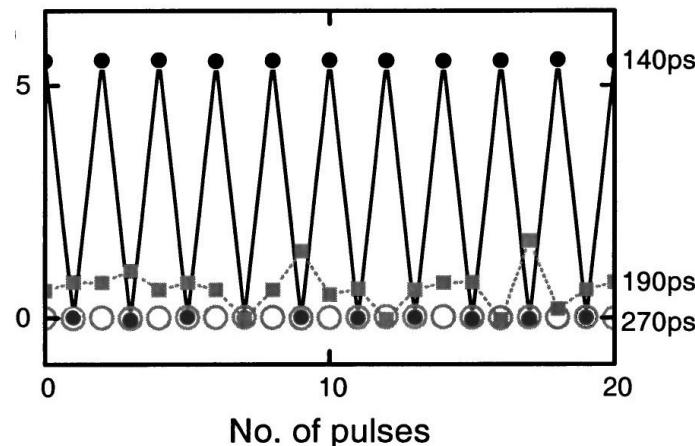
Precessional switching with **140 ps** pulses of  $\mu_0 H = 15.5$  mT pulses
