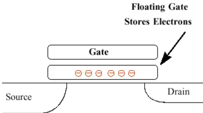
Figure 2: Single transistor flash memory cell
