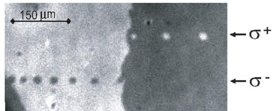
Magnetization reversal with one **40fs** circularly polarized laser pulse
