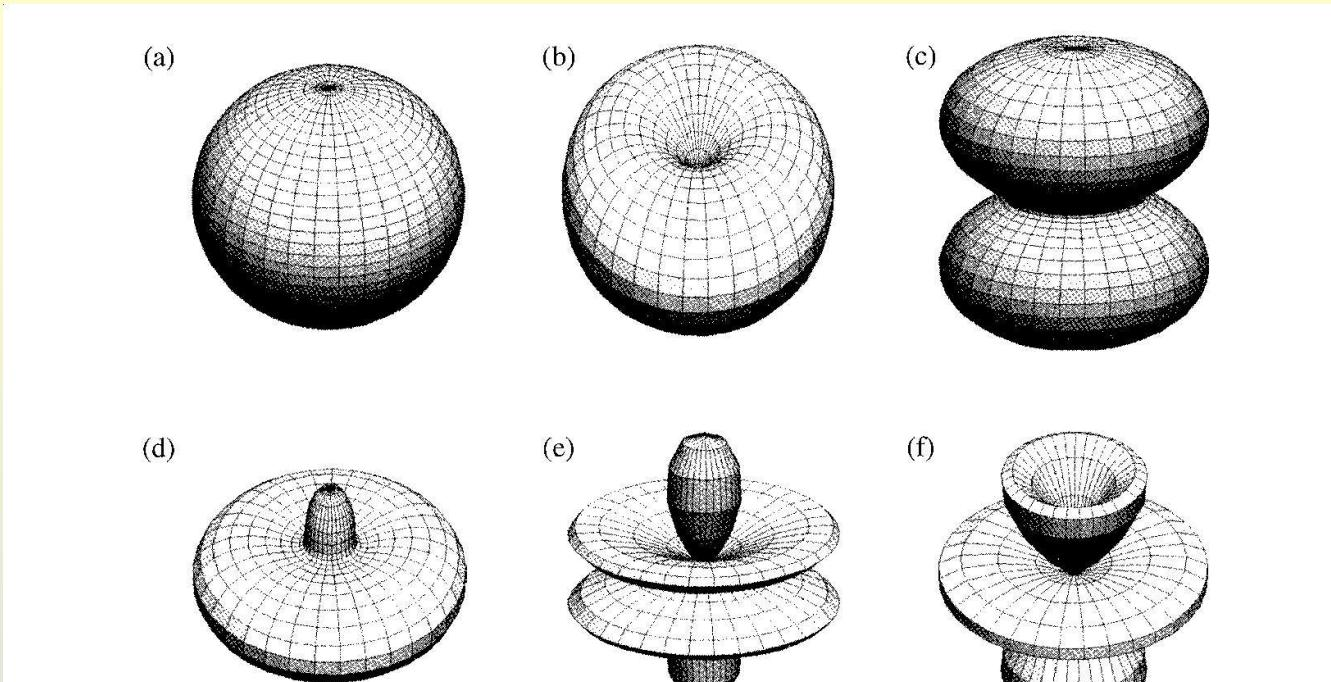
**Fig. 3.2** Uniaxial anisotropy-energy landscapes: (a) isotropic, (b) easy axis, (c) easy plane, (d) easy cone, and (e–f) sixth-order landscapes.
