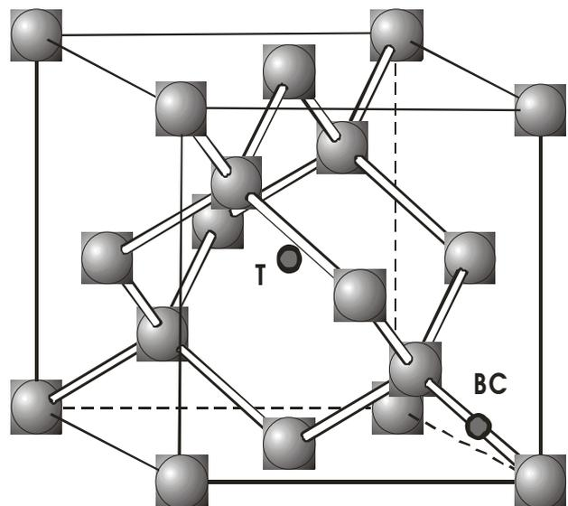
**Figure 7.** The crystal structure of silicon, showing the possible muonium (and therefore hydrogen) sites (T = tetrahedral site, BC = bond-center site).
