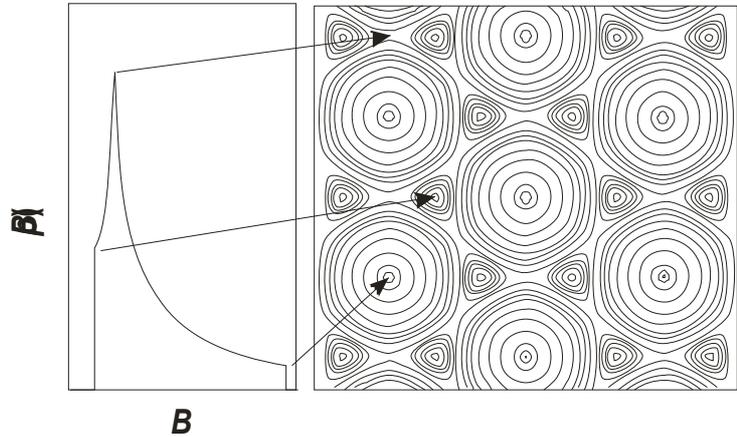
**Figure 6.** Schematic field distribution in a type-II superconductor in the mixed (vortex) state. The right-hand side of the figure represents a contour plot of the field  $B$  (from Blundell SJ (1999) Spin-polarized muons in condensed matter physics. *Contemporary Physics* 40: 175
