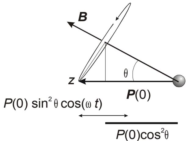
**Figure 3.** Muon-spin precession around an internal field  $B_{\mu}$  at an angle  $\theta$ . The wiggling and nonwiggling components on the polarization are schematically represented.
