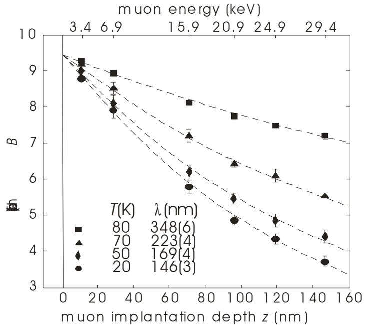
**Figure 5.** Values of the field vs. Depth measured in a high- $T_c$  sample ( $\text{YBa}_2\text{Cu}_3\text{O}_{7-\delta}$ ) for various values of temperature. The muon implantation depth is changed by tuning the kinetic energy of the muons (T.J. Jackson et al., Phys. Rev. Lett **84** (2000) 4958)
