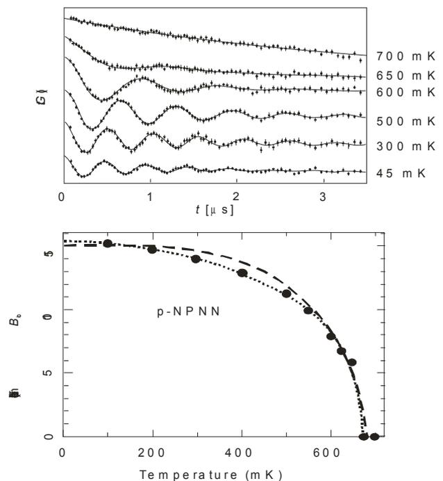
**Figure 4.** Zero-field muon-spin rotation frequency in the organic ferromagnet *p*-NPNN (from Blundell SJ (1999) Spin-polarized muons in condensed matter physics. *Contemporary Physics* 40: 175.) and temperature dependence of the local field at the muon site deduced from the observed frequency.
