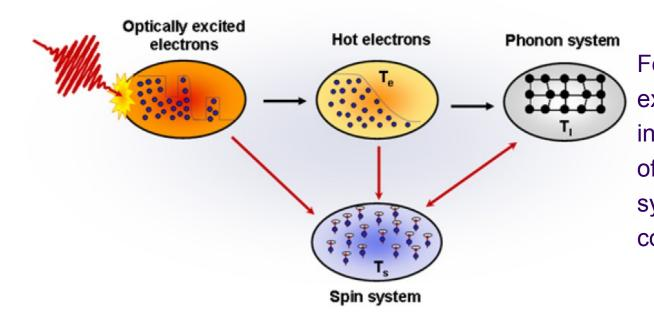
Femtosecond pump-probe experiment allows to investigate the dynamics of electron, phonon and spin systems in non-equilibrium conditions
