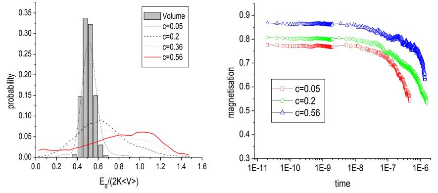
Energy barrier and magnetic relaxation calculated for conventional Co longitudinal recording medium
