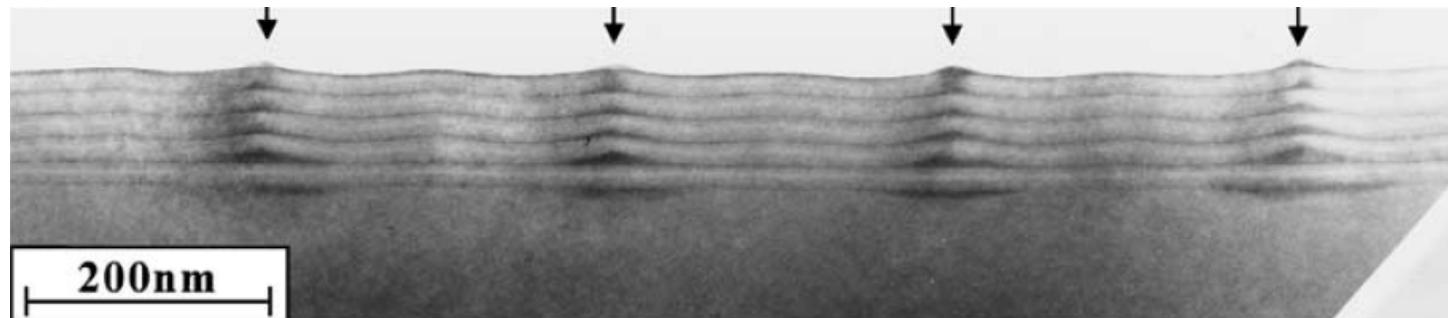
e.g. vertical alignment of InAs QDs in GaAs
