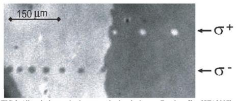
FIG.3. All-optical magnization reversal using the inverse Faraday effect [STA2007].
