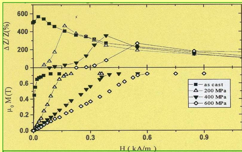
CoFeSiB amorphous wire after thermal stress-annealing inducing circular anisotropy (correlation GMI & Magnetization Curves)
