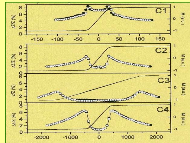
Transverse anisotropy induced by thermal field-annealing (C1,C4) and stress-annealing (C2,C3) (FeSiBCuNb Nanocrystalline)
