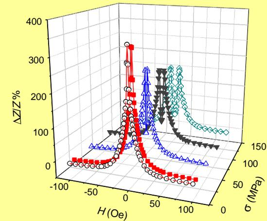
Transition from "Single Peak" to "Double Peak" by applying tensile stress (Inducing circular anisotropy)
