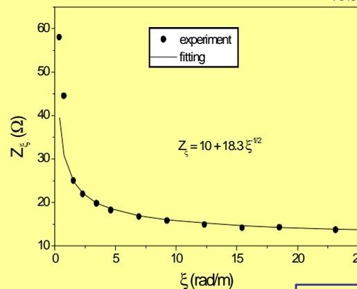
Torsion-Impedance: its fitting to a model
