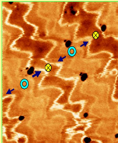
Determinating domain structure through Impedance & MFM
