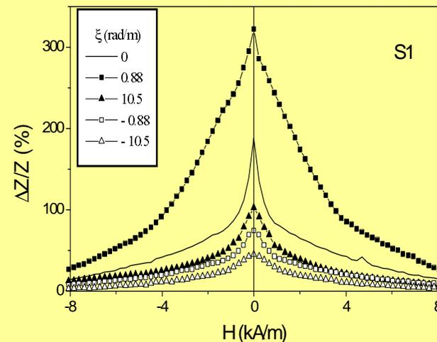
Dependence on torsion of GMI in a nanocrystalline wire  $\text{Fe}_{73.5}\text{Cu}_1\text{Nb}_3\text{Si}_{13.5}\text{B}_9$
