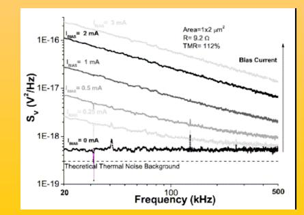
If we increase the signal to noise ratio, we expect to get high sensitivity in our magnetoresistive biosensor
