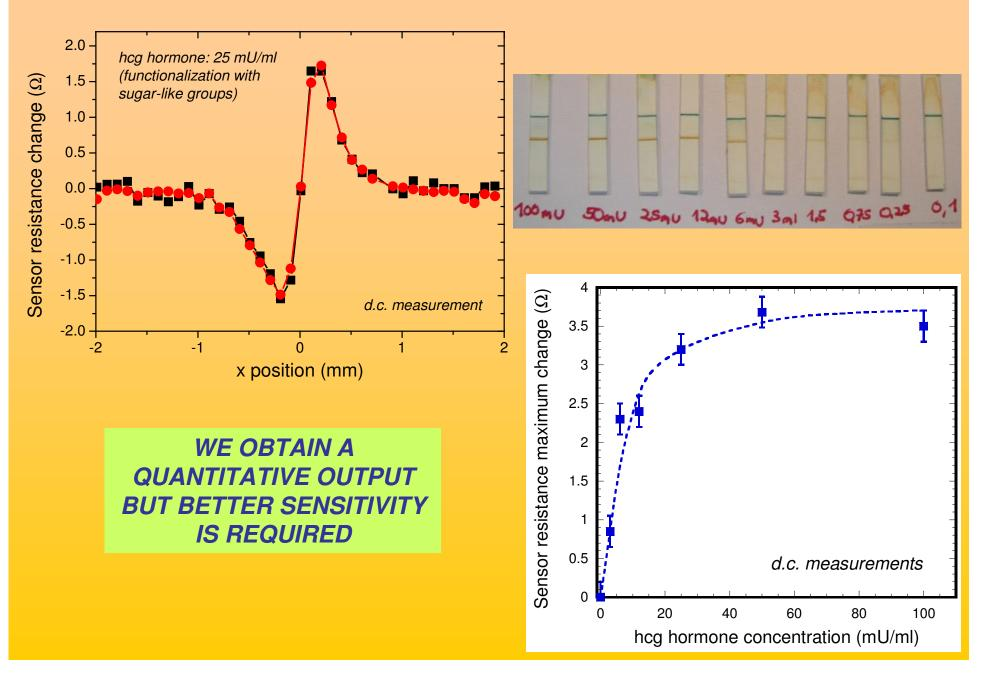
NEXT STEP: USE OF TMR SENSORS BASED ON MgO BARRIERS (MR~150%), WHICH MEANS 50 TIMES HIGHER SIGNAL, INTEGRATED ON ac WHEASTONE BRIDGES
