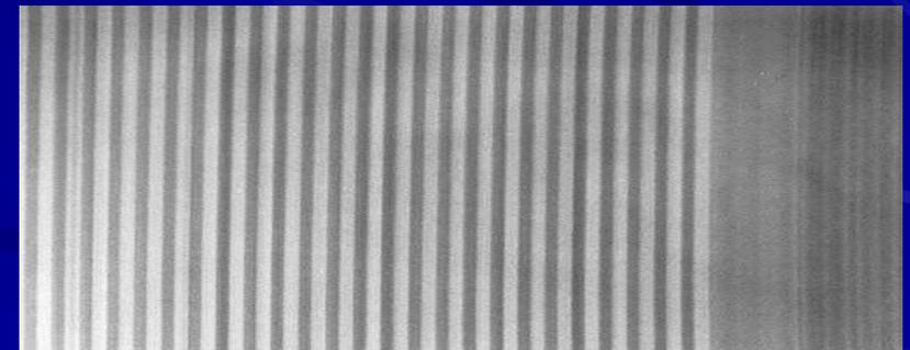
$\text{Si}_{0.76}\text{Ge}_{0.24} / \text{Si}_{0.84}\text{Ge}_{0.16}$  superlattice
