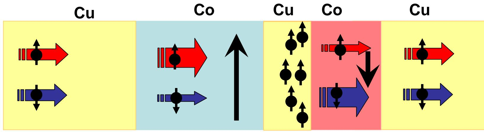
Exchange interaction between injected polarized  $e^- \uparrow$
