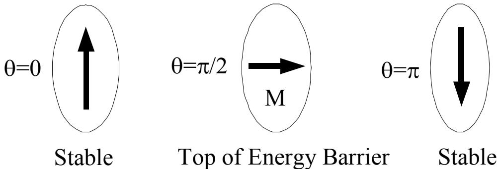
Stable states of the remanence of a magnetic particle. Thermally induced reversal of the particle magnetisation is possible when its volume becomes small enough. This phenomenon is called superparamagnetism and is one of physical limits that is being “pushed back” to improve recording density. Coupling to artificial antiferromagnetic layers has recently allowed the use of particles smaller than the superparamagnetic limit !
