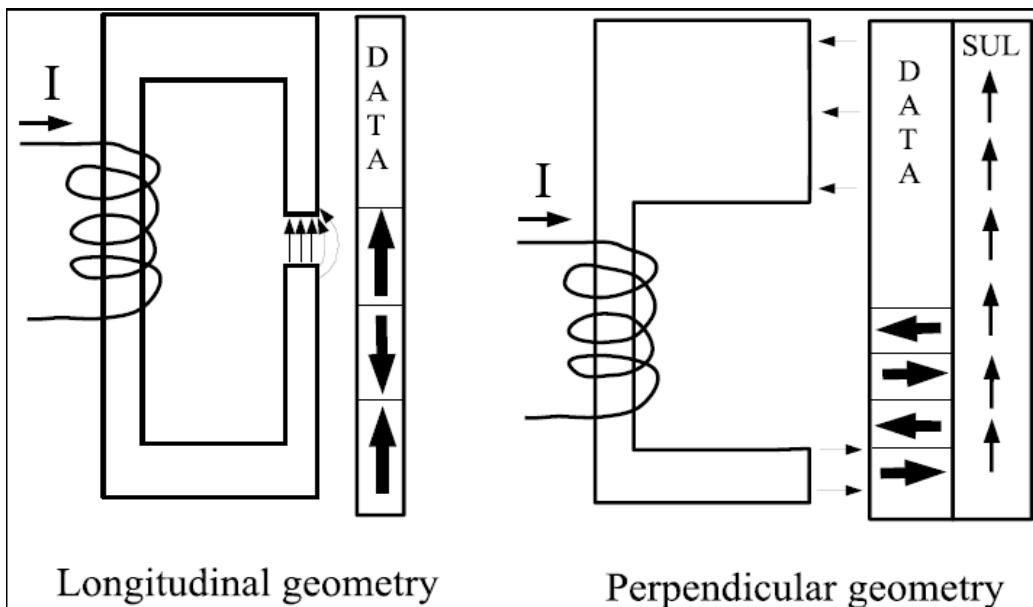
Tapes, floppies and hard disks traditionally used in-plane magnetisation (longitudinal geometry). Since 2006, perpendicular magnetisation is being used in hard disks as a way to improve density. It is a major technological leap, since new media with out of plane anisotropy had to be developed and must include magnetically soft underlayers to guide the magnetic flux. Write heads and read heads had also to be redesigned for this new geometry.
