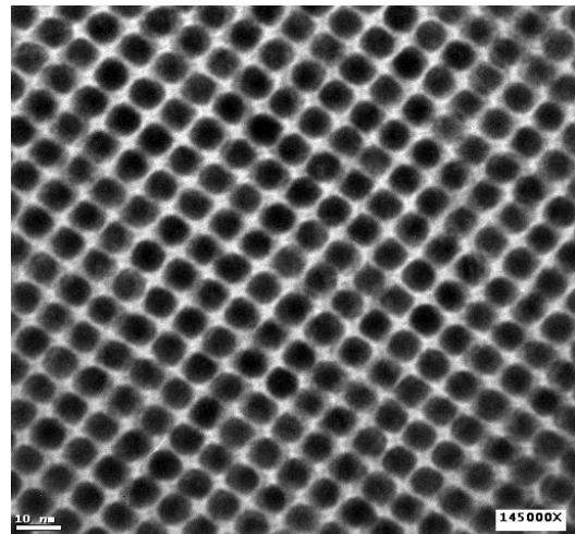
To improve recording density, small particles with very narrow size distribution have to be synthesised. New materials such as high anisotropy FePt L1<sub>0</sub> are candidates. The following aim is to spatially organise the particle positions (lithography, self organisation...) and eventually to use only one particle / magnetic bit. (images from D. Weller (Seagate) see S. Sun, C. Murray, D. Weller, L. Folks, A. Moser, Science, 287, 1989 (2000))
