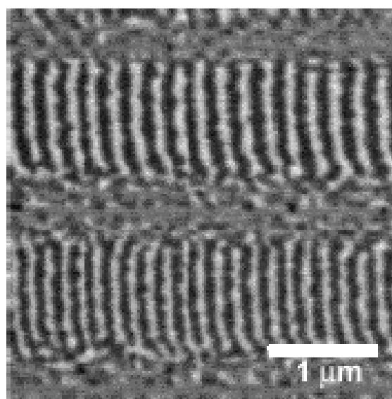
MFM image of recorded tracks (longitudinal recording). One magnetic bit contains roughly 100 magnetic grains (cobalt based) so that the information is stable against losing (i.e. reversing) a few magnetic grains. The way information is coded and physically written gives also possibilities to improve density.
