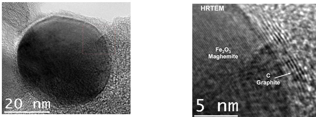
HRTEM images of carbon coated magnetic nanoparticles produced by arc discharge. As corresponds to a lighter element, C appears with a lighter contrast compared to Fe.
