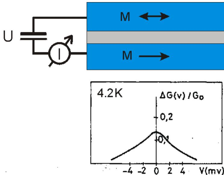
Fig. 2. Relative conductance  $(\Delta G/G)|_{V=0}$  of Fe-Ge-Co junctions at 4.2 K.  $\Delta G$  is the difference between the two conductance values corresponding to parallel and antiparallel magnetizations of the two ferromagnetic films.
