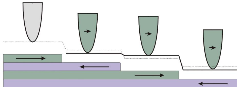
With non-magnetic W tips, the standard step height of 1.4 Å is observed
