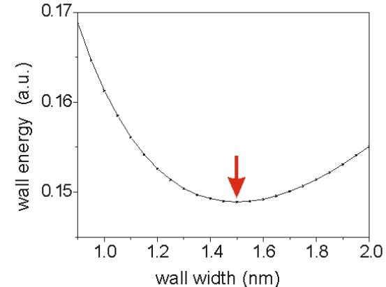
Sum of exchange and anisotropy energy of 20° wall shows minimum at 1.5 nm width.
