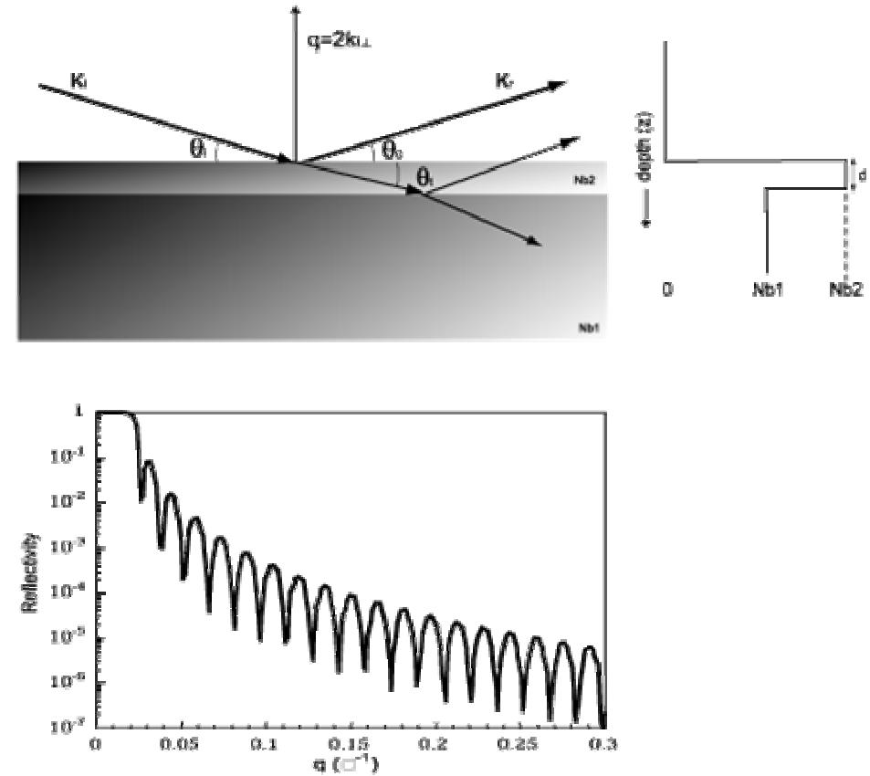
Specular reflectivity can derive the scattering length density and absorption as a function of depth
