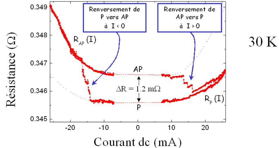
Pillar cross-section :  $200 \times 600 \text{ nm}^2$
