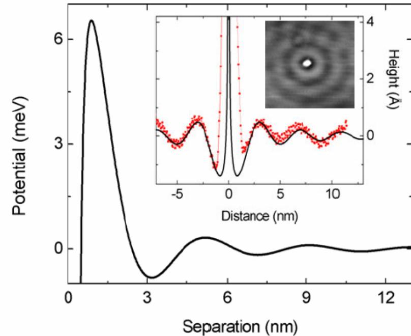
**Figure 9.** Calculated two-body interaction potential of Ce adatoms on Ag(111) (equation (2)). Inset:  $21 \times 21 \text{ nm}^2$  STM topography of a standing-wave pattern around an isolated Ce adatom on Ag(111) at 3.9 K ( $U_s = -3 \text{ mV}$ ,  $I_s = 19 \text{ pA}$ ). Topographic cross-section (dots) and fit using equation (1) (solid curve) as a function of distance from a single Ce adatom.
