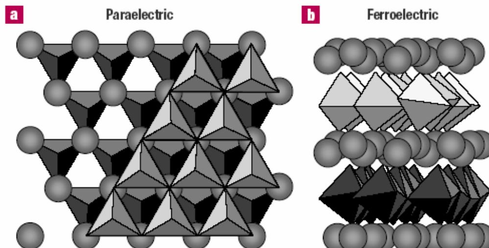
**Figure 1** The crystal structure of  $\text{YMnO}_3$  in the paraelectric and ferroelectric phases. The trigonal bipyramids depict  $\text{MnO}_5$  polyhedra and the spheres represent Y ions. **a**, The stacking of two consecutive  $\text{MnO}_5$  layers and the sandwiched Y layer, looking down the  $c$  axis in the paraelectric phase. **b**, A view of the ferroelectric phase from perpendicular to the  $c$  axis, showing the layered nature of  $\text{YMnO}_3$ .
