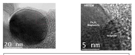
HRTEM images of carbon coated magnetic nanoparticles produced by arc discharge. As corresponds to a lighter element, C appears with a lighter contrast compared to Fe.
