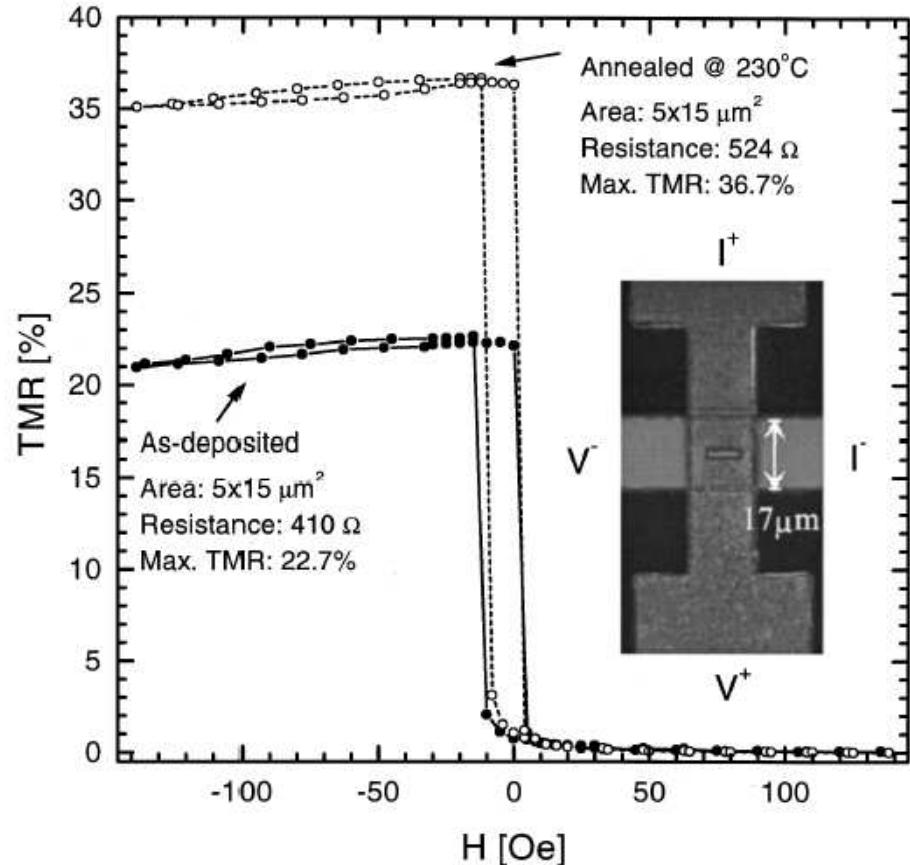
FIG. 1. Tunneling magnetoresistance vs field for an as-deposited spin tunnel junction, and for the same junction after consecutive anneals up to 230 °C. In the inset, the four-probe measuring scheme is illustrated using an optical microscope picture of the junction.
