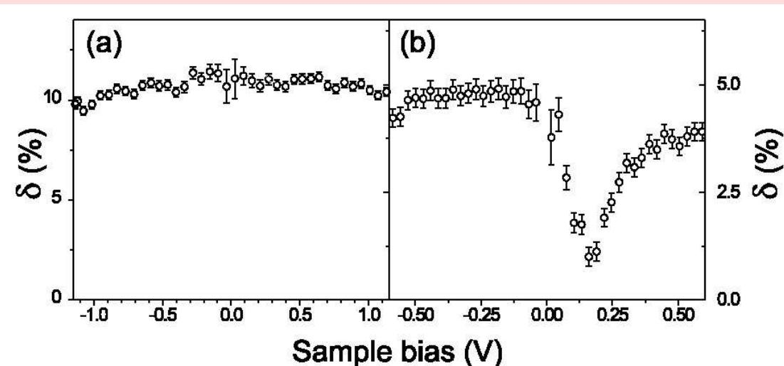
FIG. 1. Tunnel magnetoresistance  $\delta$  and its error of a clean Co(0001) surface vs bias voltage  $U$ , obtained with a magnetic tip stabilized at 1 V, 1 nA (a) and at 100 mV, 1 nA (b).
