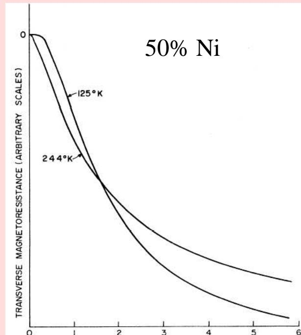
FIG. 5. Transverse magnetoresistance vs applied magnetic field for 50 vol% Ni.
