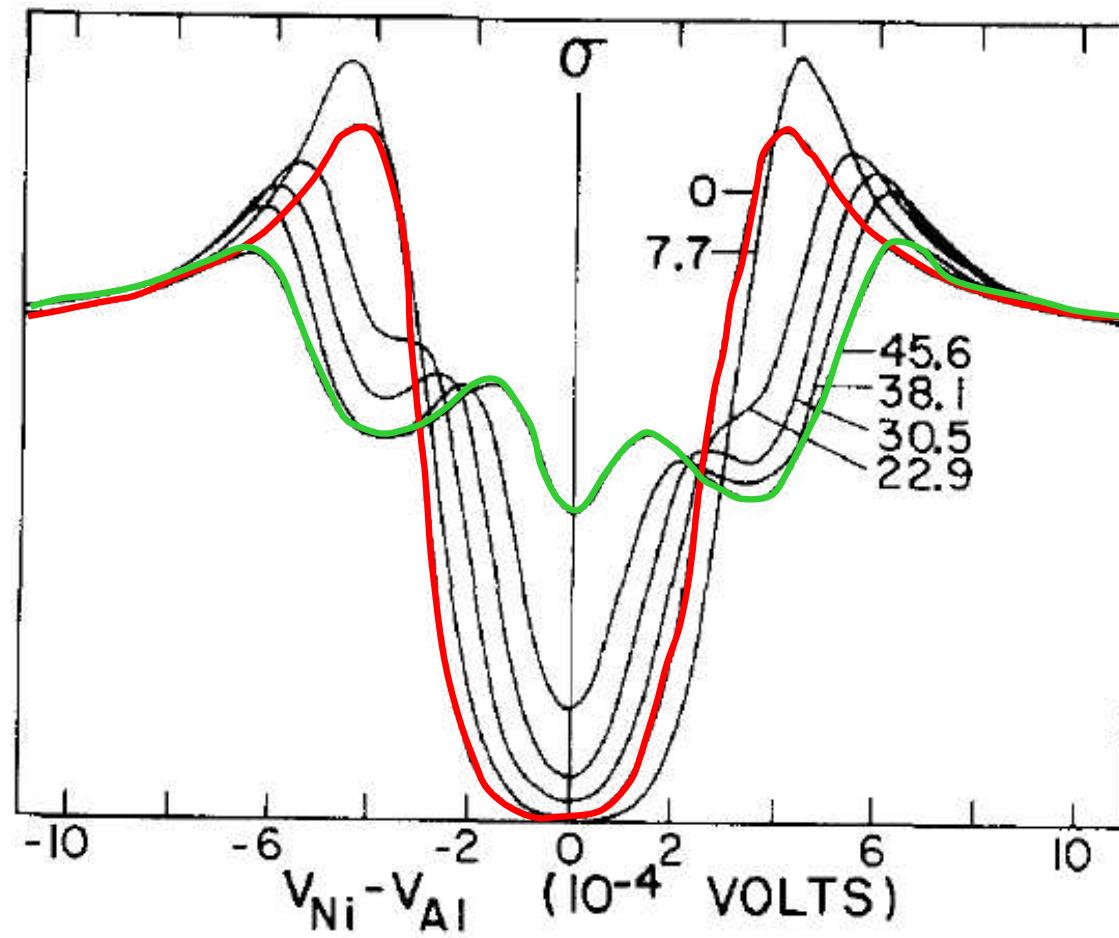
Fig. 1 Measured conductance vs voltage of an Al-Al<sub>2</sub>O<sub>3</sub>-Ni tunnel junction for several values of the magnetic field H(kOe).
