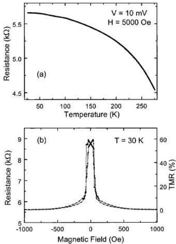
FIG. 2. Transport studies for a Fe(001)/MgO 20 Å(001)/FeCo(001) tunnel junction of diameter 10  $\mu\text{m}$ : (a) resistance vs temperature at  $V=10 \text{ mV}$  and  $H_{\text{app}}=5000 \text{ Oe}$ ; (b) resistance and TMR vs magnetic field at  $V=10 \text{ mV}$  and  $T=30 \text{ K}$ .
