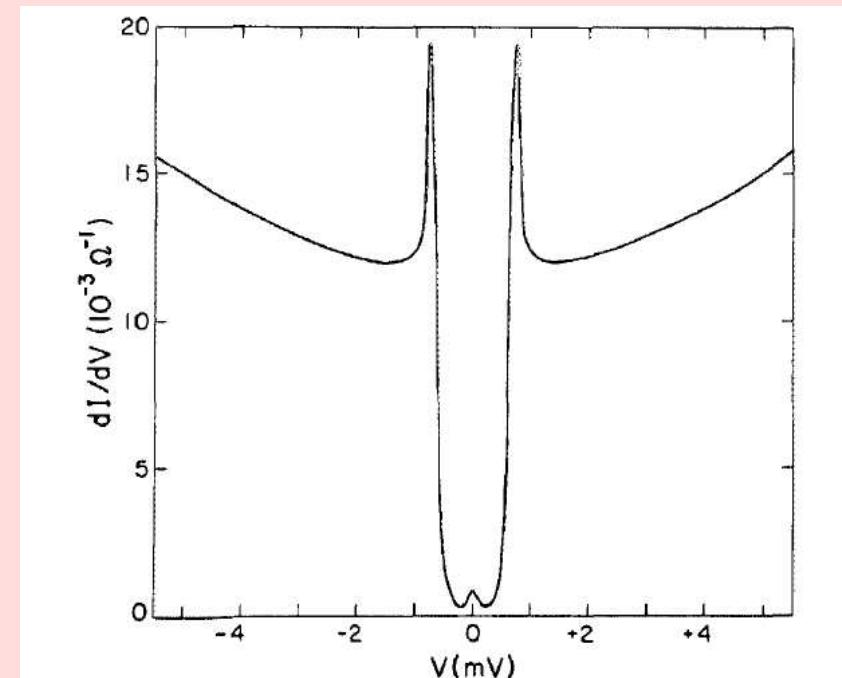
FIG. 6.  $dI/dV$  vs  $V$  for an Al/a-Ge/Al junction at 1.2 K, when the thin aluminum is superconducting. The superconducting energy gap is clearly visible. The large near-parabolic background is the result of the small effective barrier height. The small peak at zero voltage is characteristic of tunneling between identical superconductors at finite temperature.
