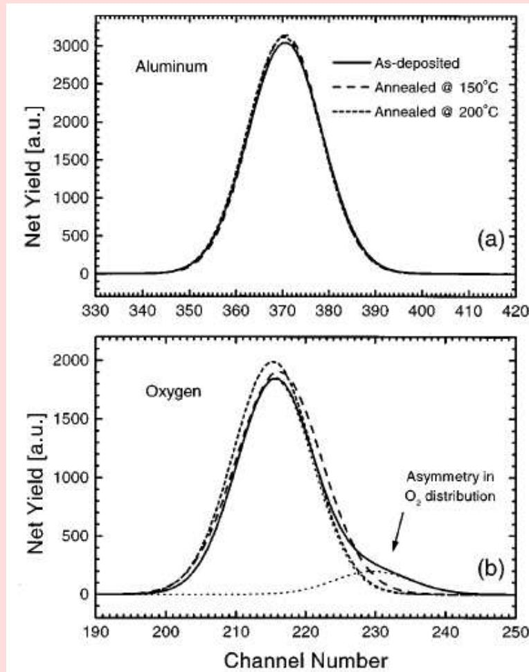
FIG. 5. Gaussian curve fits to the aluminum (a) and oxygen (b) peaks obtained by Rutherford backscattering analysis, for as-deposited junctions, and for junctions annealed at 150 and 200 °C.
