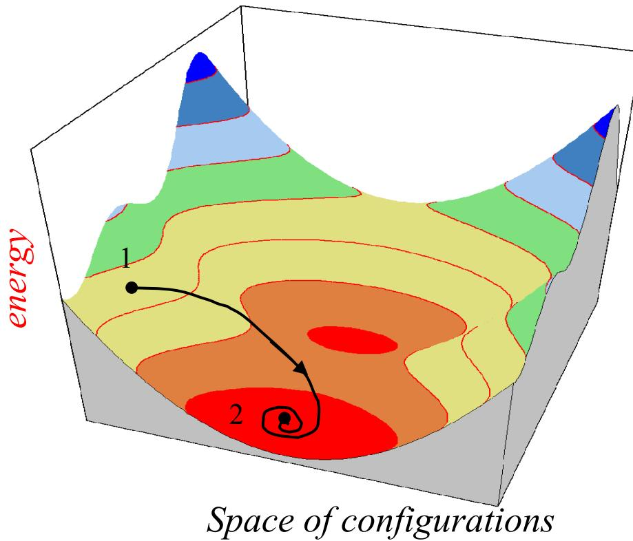
magnetization trajectory between two magnetic states
