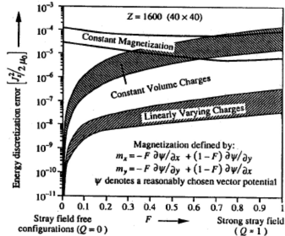
Fig. 1. Energy discretization error for configurations as defined in the inset where the parameter  $F$  generates a completely stray-field-free configuration for  $F = 0$  and configurations of strong field for  $F = 1$ . The bands indicate the range of results obtained for many computer experiments.
