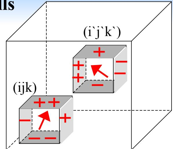
$$E_D = \frac{\mu_0}{8\pi} \iint_S \iint_S \frac{\sigma_m(\vec{r}) \sigma_m(\vec{r}')}{|\vec{r} - \vec{r}'|} dS dS' = \frac{1}{2} \mu_0 M_s^2 \sum_{I=1}^{N_{cells}} \vec{m}_I \cdot \langle \vec{H}_D \rangle_I V_{cell}$$
