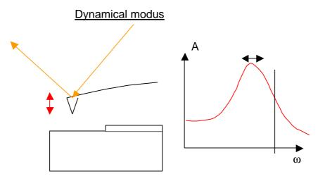
Cantilever is excited to vibrations near to its eigenfrequency; additional external force gradients change the effective force constant of the cantilever and so its resonance frequency. A feedback controls either the amplitude or the phase shift of the vibration.
