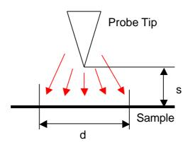
Resolution is not longer diffraction-limited; limitation due to geometry and type of interaction
