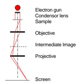
Very thin (electron transparent) samples. Image appears due to interaction of the electron beam with the sample (absorption, scattering, phase shift). Maximum lateral resolution ~ 0.1 nm. Information about internal structure of the transmitted sample.
