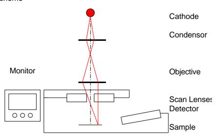
Measured is the yield of secondary electrons at each scanned point. Lateral resolution limit 1 ... 10 nm. Imaged are the surface and near-surface properties (there are also detected X-Rays, photons, backscattered and Auger electrons).
