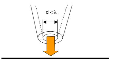
Subwavelength aperture; propagating and evanescent parts of the electromagnetic field.
