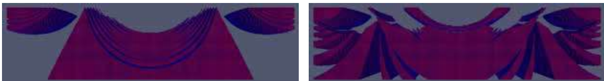
Figure 1: Exemplary result for the optimum magnetic shape with a local optimization algorithm (left) and our presented hybrid optimization algorithm (right). The found optimum of the latter variant results in a 75.5% lower value of the given objective function and presents therefore a significantly better optimum with the same depth of local optimization steps.
