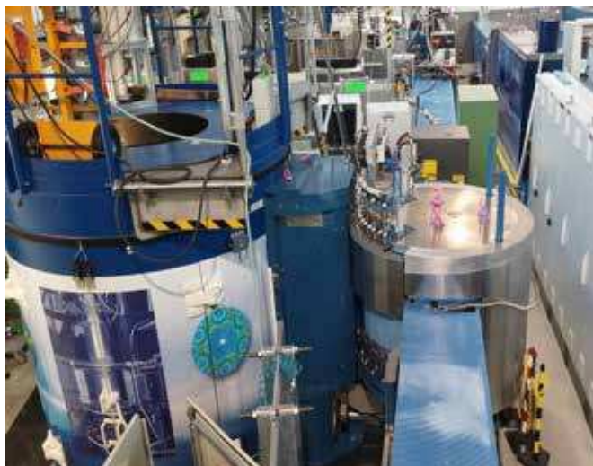
Figure 1: Picture of the DNS instrument, with the secondary spectrometer to the left and monochromator housing and neutron guide to the right.
