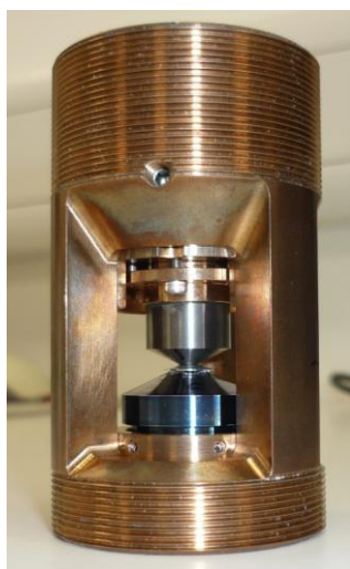
Fig. 1 Photograph hybrid-anvil-type high-pressure cell.[2]
