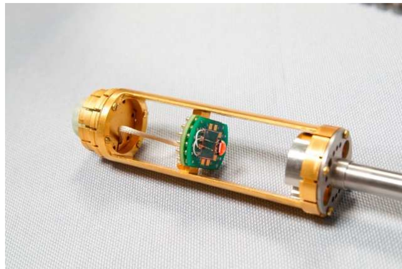
Illuminated sample mounted to MFP ready to go for variable magnetic field and temperature
