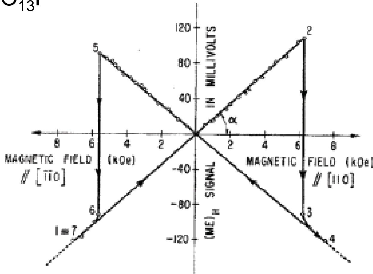
FIG. 4. Example of a quadratic magnetoelectric hysteresis loop with  $H$  along  $\pm[110]$  and  $P$  along  $[001]$  at  $46^\circ\text{K}$ . After annealing as in Fig. 3.
