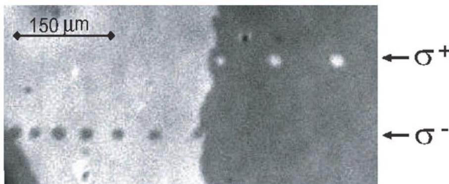
FIG.3. All-optical magnetization reversal using the inverse Faraday effect [STA2007].
