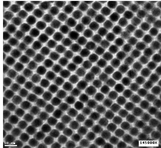
To improve recording density, small particles with very narrow size distribution have to be synthesised. New materials such as high anisotropy FePt L1<sub>0</sub> are candidates. The following aim is to spatially organise the particle positions (lithography, self organisation...) and eventually to use only one particle / magnetic bit. (images from D. Weller (Seagate) see S. Sun, C. Murray, D. Weller, L. Folks, A. Moser, Science,287,1989 (2000))
