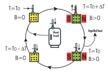
Figure 1 Schematic representation of a magnetic-refrigeration cycle, which transports heat from the heat load to the ambient. Left and right depict material in low and high magnetic field, respectively.
