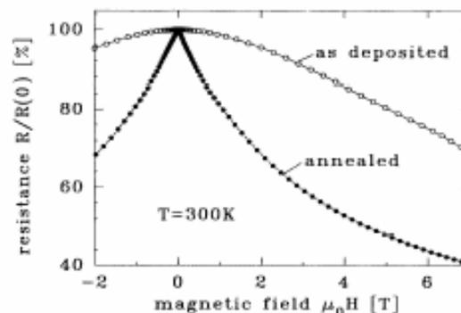
FIG. 3. Resistivity versus field curves for the as-deposited sample ( $T_S = 600^\circ\text{C}$ ) and after annealing at  $T_A = 900^\circ\text{C}$  for 12 h, measured at  $T = 300\text{ K}$ .
