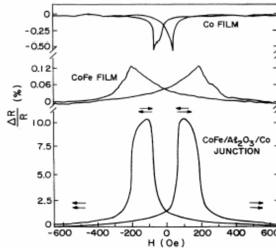
FIG. 2. Resistance of CoFe/Al<sub>2</sub>O<sub>3</sub>/Co junction plotted as a function of  $H$  in the film plane, at 295 K. Also shown is the variation in the CoFe and Co film resistance. The arrows indicate the direction of  $M$  in the two films (see text).
