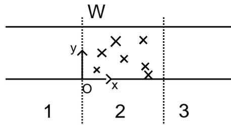
FIG. 2: In this ideal wire, the part 1 and 3 are ballistic while all the scattering takes place in region 2. The electrons are confined in the region  $0 \leq y \leq W$  and the wire is attached to two ideal reservoirs.
