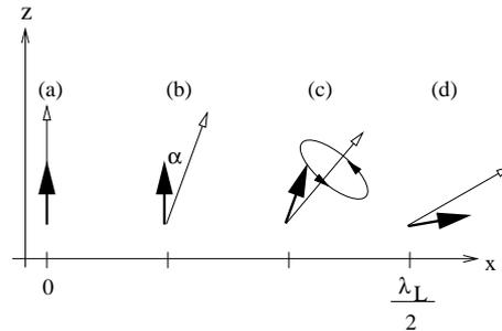
FIG. 5: Competition between the rotation of the magnetization and Larmor precession in a domain wall. The thick arrow stands for the electron spin while the thin one stands for the magnetization.
