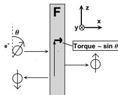
FIG. 3: Polarized electrons incident on a single magnetic layer.
